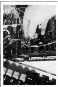
Connect the control wires
